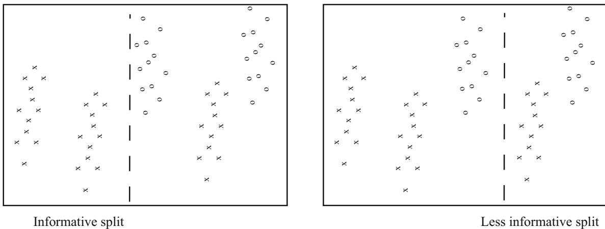
Fig. 11.8 Two possible splits of a pool of training data. Positive data is represented with an ‘x’, negative data with a ‘o’. Notice that if we split this pool with the informative line, all the points on the left are ‘x’s, and two-thirds of the points on the right are ‘o’s. This means that knowing which side of the split a point lies would give us a good basis for estimating the label. In the less informative case, about two-thirds of the points on the left are ‘x’s and about half on the right are ‘x’s—knowing which side of the split a point lies is much less useful in deciding what the label is
