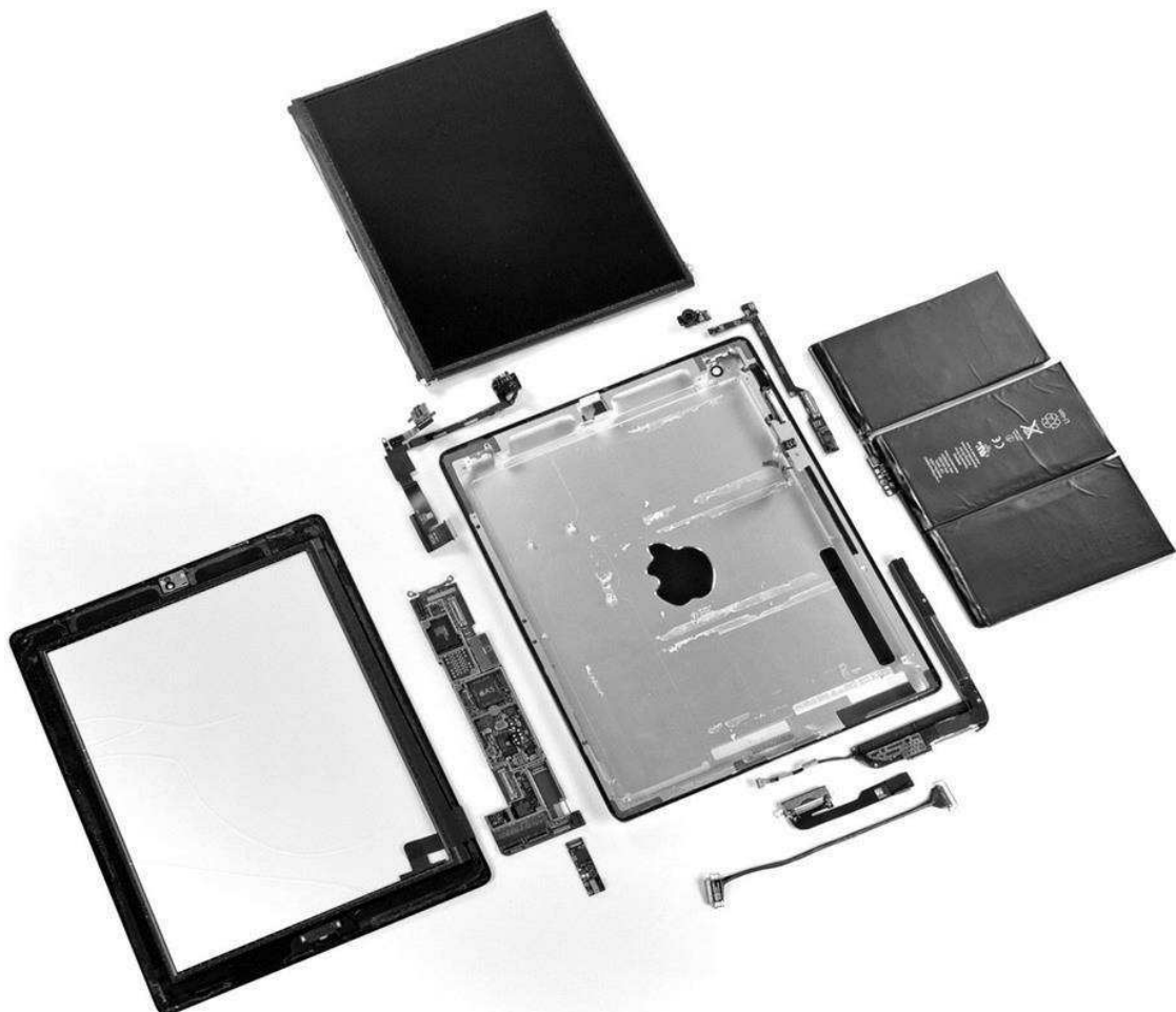
FIGURE 1.7 Components of the Apple iPad 2
