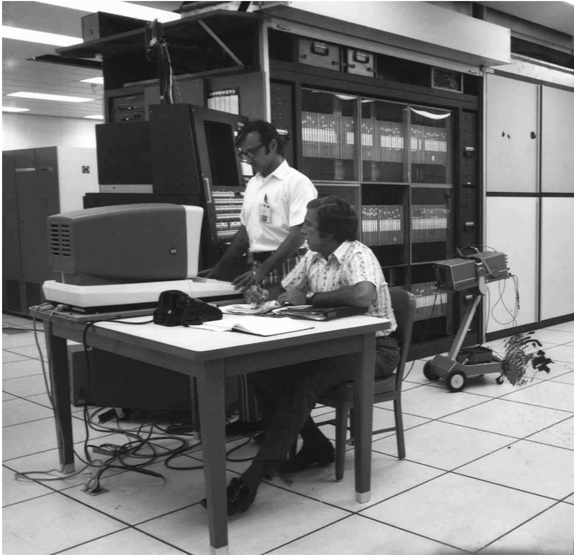
FIGURE E6.15.1 The Illiac IV control unit followed by its 64 processing elements.
